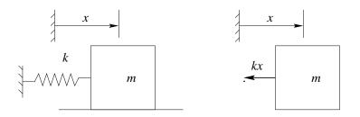
From the free body diagram (F.B.D.) of the mass, we can see that the only force acting on the mass is the spring force provided that there is no external force. Using Newton's laws, we can easily obtain the dynamic equation:
